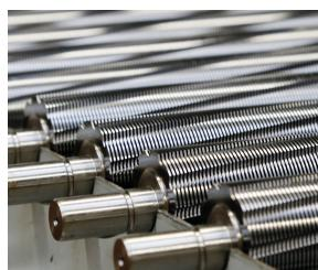
The induction-hardened, solid steel cutting rollers with a lifetime warranty can easily cope with staples and paper clips and guarantee durability.
